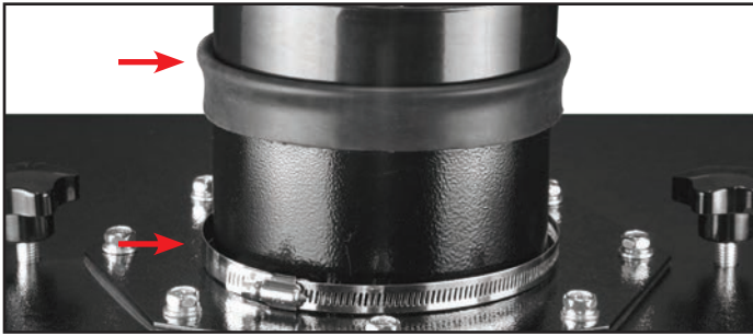
2. Install the elastic sealing ring on the base then fold half. Install hose clamp and stay loose on the base.
