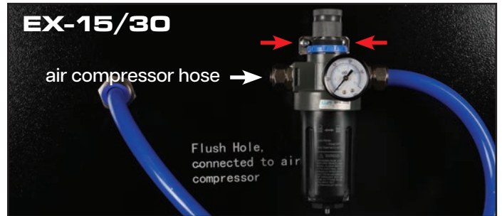
9. Take out the oil-water separator from the front storage. Install the oil-water separator on the side of the unit then connect the gas source. (This is for reverse blowing function, clean dust method)
