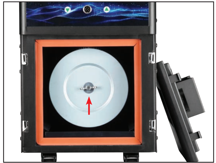
2. Unlock the knobs on top of the filter cartridge to take out the filter.
