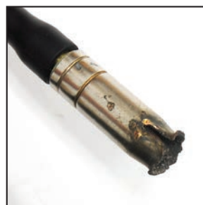
Build up of spatter can cause damage to nozzle and tip
