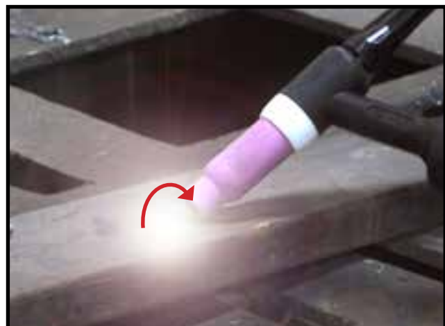
4 Now rotate the Gas Cup in the reverse direction to lift the Tungsten electrode from the work piece to create the arc.
