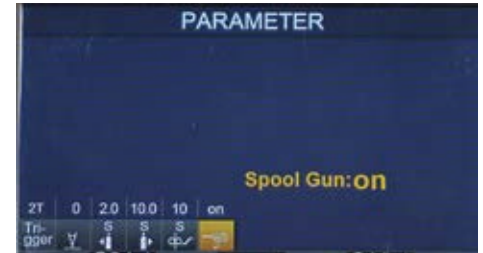
Spool gun setting in MIG manual
