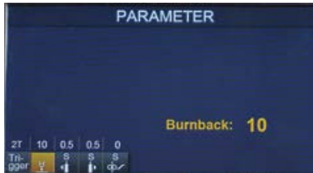
Adjustable burnback control in MIG
