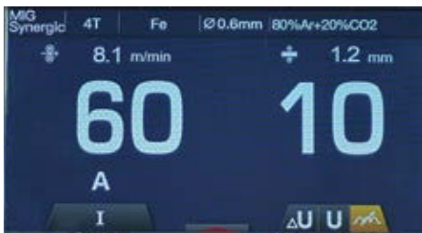
Inductance adjustment in MIG
